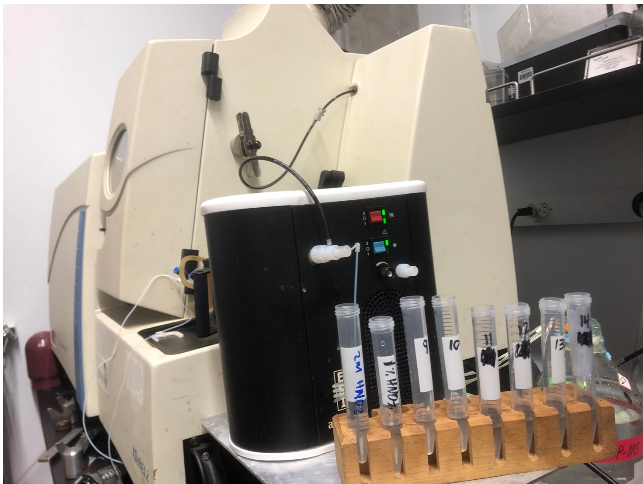
Attachment 12. Photo of the NAU Thermo X2 quadrupole ICPMS and ESI APEX HF sample introduction system used in the study of the April 6, 2024 air filter samples; photo taken on May 3, 2024 on the day following analyses of the samples from the air filter study
